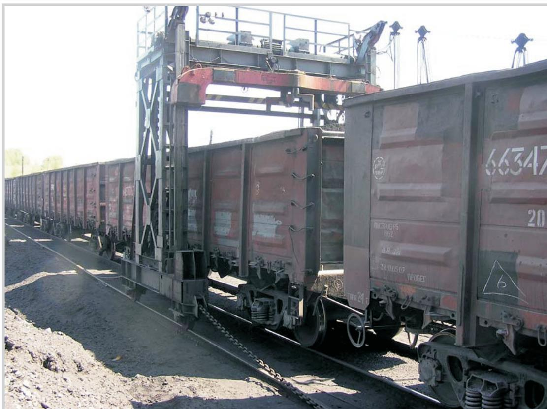
The machine is applied for periodic hauling of car trains of any sequence, consisting of four, six and eight open box cars with total mass – up to 2000 tones to the loading and unloading points of mines and processing plants.
