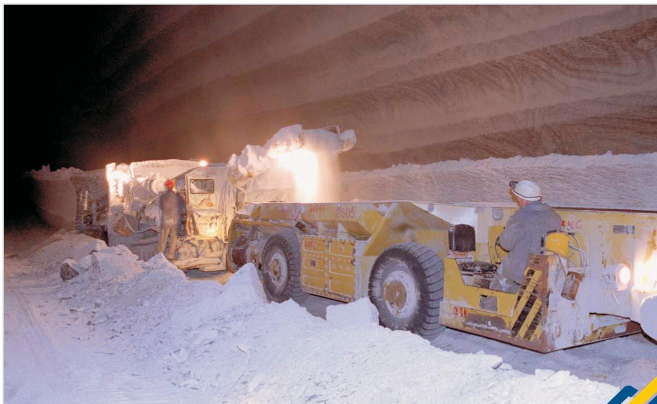
The machine is applied for transportation of mined material in underground mines that are gas (methane) – hazardous and dusty. The car is manufactured in two versions: for potash mines and coal mines. Electrical equipment execution – mine, blast-proof. The car for coal mining has undergone certain modifications as follows:
